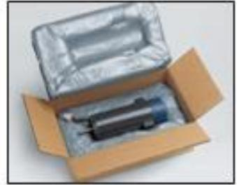
1. Instapak foam is dispensed into a carton lined with high-strength Instamate film.
